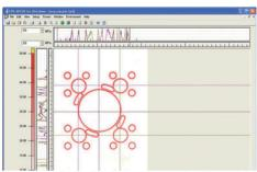
Pressure distribution on a line passing through a specified point is shown on a line praph.
